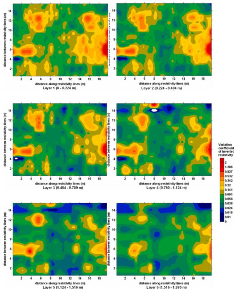
Figure 1. The variation coefficient of the inverted resistivity data at six layers from the surface to approximately 2 meter, at the Filborna landfill.
