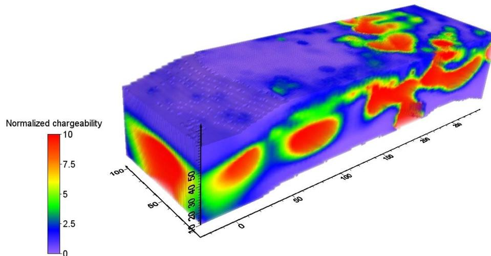
Figure 2. 3D model from part of Filborna waste deposit; a) resistivity, b) normalised IP.
