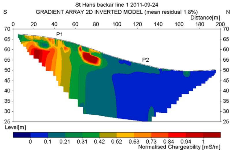
Figure 1. 2D inverted models from St Hans Backar; a) resistivity, b) normalised IP. P1 and P2 marks positions of test pits.
