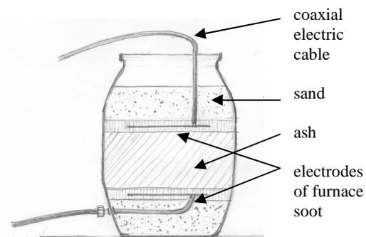
In the laboratory 100 litre drums were filled with the same materials as in the field and compacted. Two electrodes were placed above and below the compacted ash as shown in the Figure.
