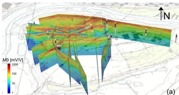
**Figure 2** Gathered 2-D sections in chargeability with superimposed boreholes, allowing a 3-D characterization of the landfill area.
