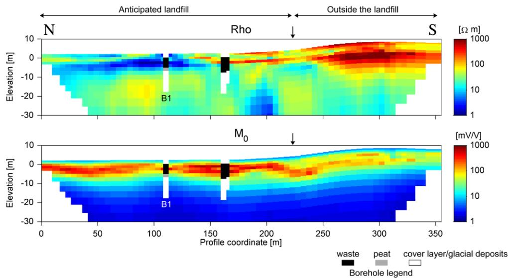
**Figure 1** Results from a 1-D Laterally Constrained Inversion for a section in-between the landfill area, with superimposed boreholes. Top: resistivity, bottom: chargeability  $M_0$ .
