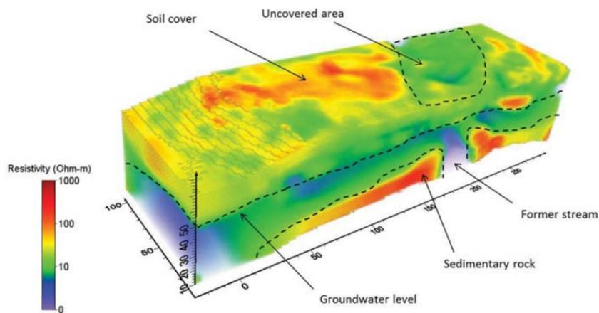
The figure to the left shows the inverted and interpreted resistivity model. The sedimentary rock, the expected ground water level and the soil cover is visible. A zone with low resistivity at the surface is evident in the right part of the model, where the cover layer is missing. At length coordinate 200 m a distinct low resistivity zone is visible, which corresponds to the position of a former stream below the landfill, indicating contaminant leachate migrating into the former stream.
