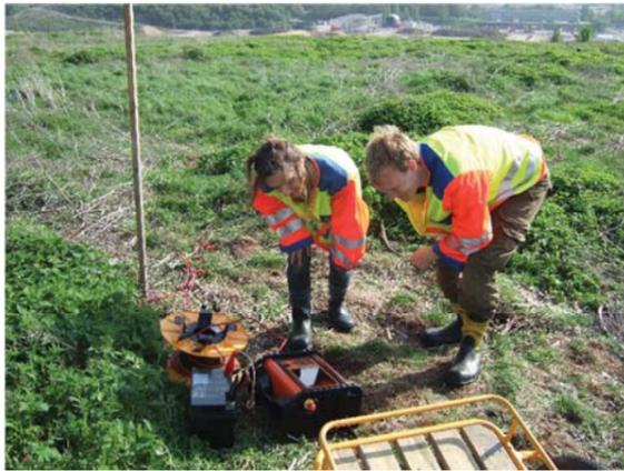
Data acquisition was made with an ABEM Terrameter LS with 12 measuring channels, using 300 m long layouts with 5 m electrode take-out spacing. A total of 11 lines 300 m long and spaced 10 m were measured in one field week, resulting in 17680 resistivity-IP data points on a total of 3300 m of profile. An expanded multiple gradient array was employed. Data were inverted with Res3dinv using L1-norm (robust) inversion.
