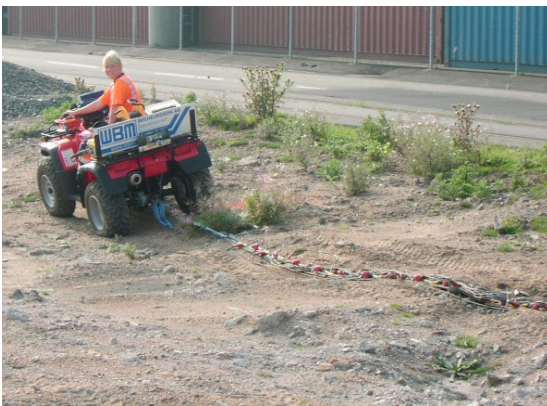
Data acquisition with a towed landstreamer.
