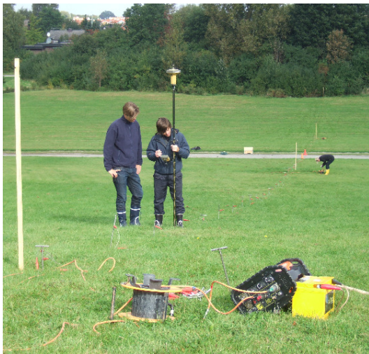
Geoelectrical data acquisition and differential GPS positioning
