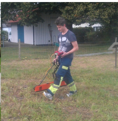
Surveying with EM38.
