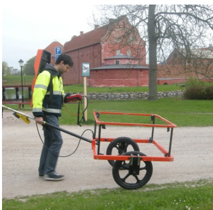
Surveying with EM61.
