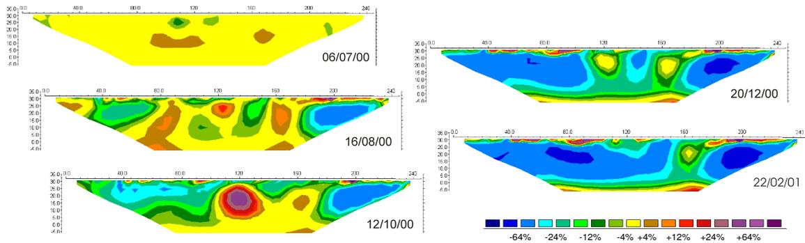
Figure 1. Sample of results from the time-lapse electrical imaging. Percentage change in resistivity recorded over the landfill, where a decrease in resistivity indicates an increase in moisture content and an increase in resistivity indicates a decrease in moisture content.
