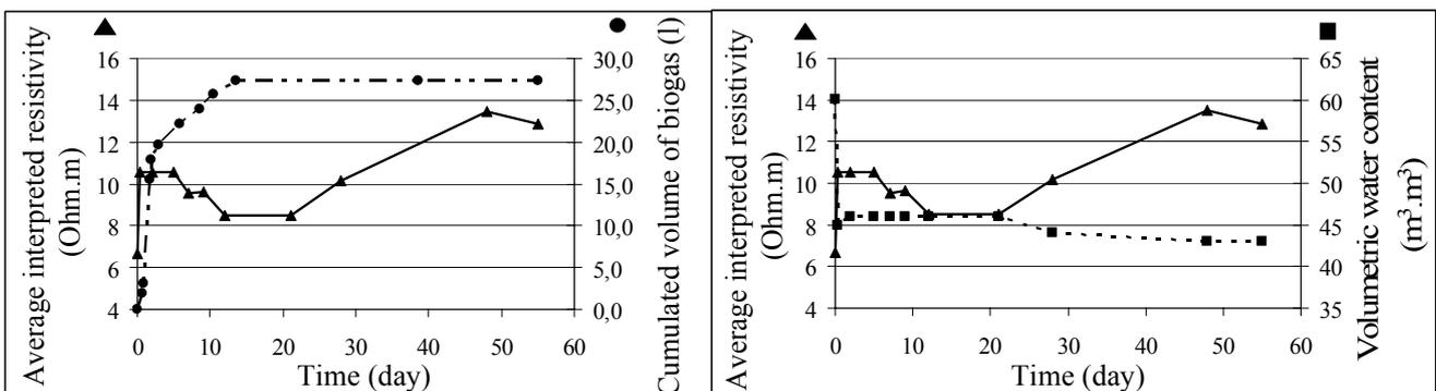
Figure 1: Average resistivity evolution according to biogas production and moisture variation
