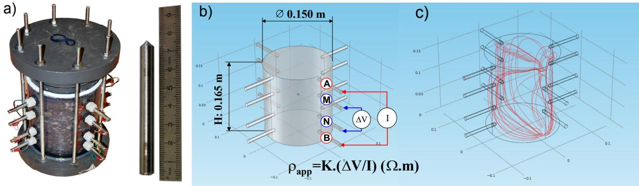
Figure 1: a) Test cell and electrodes; b) Electrical resistivity measurements (AB, current injection electrodes; MN electric potential electrodes); c) Current density
