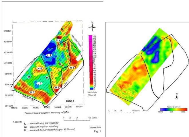
Figure 1. Results of CMD 4 (left) and large-scale resistivity (right) at the uppermost layers showed good correlation.
